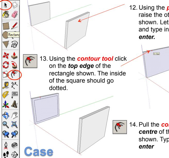
12. Using the *push pull tool* raise the other rectangle shown. Let go of the mouse and type in *250 and press enter.*
