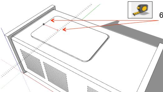
63. Use the *tape measure* tool and draw a guideline in from the left hand side edge shown. Type in 90 and press enter
