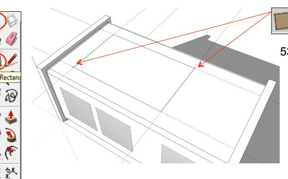
54. Use the *rectangle tool* to start drawing a square from the bottom left hand corner of the last rectangle you have just drawn. Type in 20, 20 and press
