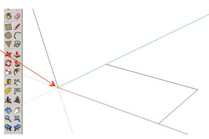
6. Let go of the mouse and start typing **580, 300** and then **press enter**. These sizes will appear in the bottom right hand corner shown.
