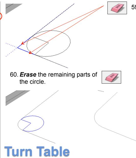
59. Use the **eraser tool** to erase the corners so you are left with a radius as shown
