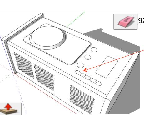
92. Use the eraser tool to erase the outside edge contours shown on the rectangles.
