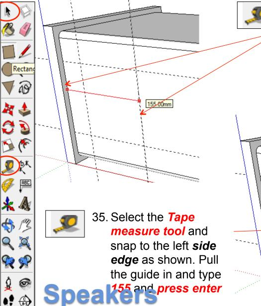
34. Select the *Tape measure tool* and snap to the left *side edge* as shown. Pull the guide in and type *155* and *press enter*
