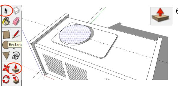
67. **Select** the **push pull tool**. Pull the circle up and type 10 and press enter.
