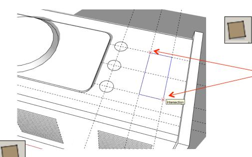
85. Using the *rectangle tool* click on the *intersection* where two dotted guidelines meet in the *top left hand corner*. Pull the rectangle down to the *bottom right hand corner intersection* shown.
