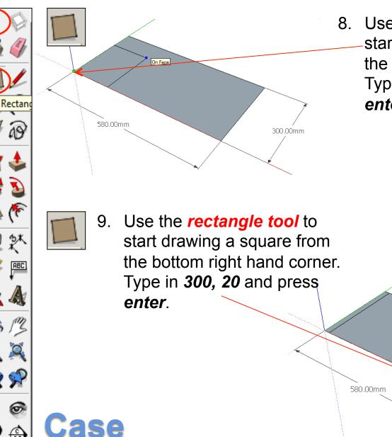
8. Use the *rectangle tool* to start drawing a square from the bottom left hand corner. Type in 300, 20 and press enter.
