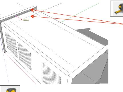
51. Use the *tape measure tool* and draw a guideline in from the left hand side edge shown. Type in *60* and *press enter*
